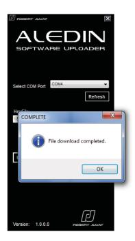
When done uploading, click OK, when the "File download completed" dialogue is shown. The 4 LEDs on the Uploader will flash once and then resume the chase.
